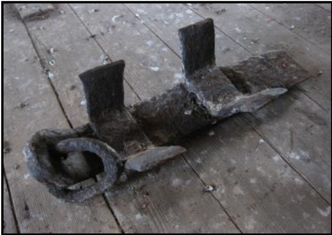
The iron emergency brake used by a stage coach or heavy wagon for descending steep hills.
